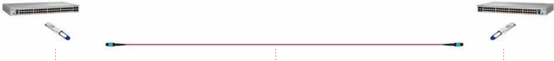
100G-QSFP MM 850nm SFP MPO patch cord 100G-QSFP MM 850nm SFP
